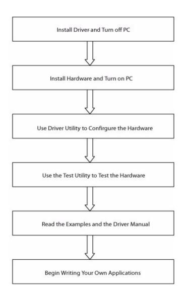
Figure 1.1: Installation Flow Chart
