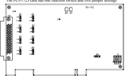
The PCI-1723 card has one function switch and five jumper settings
